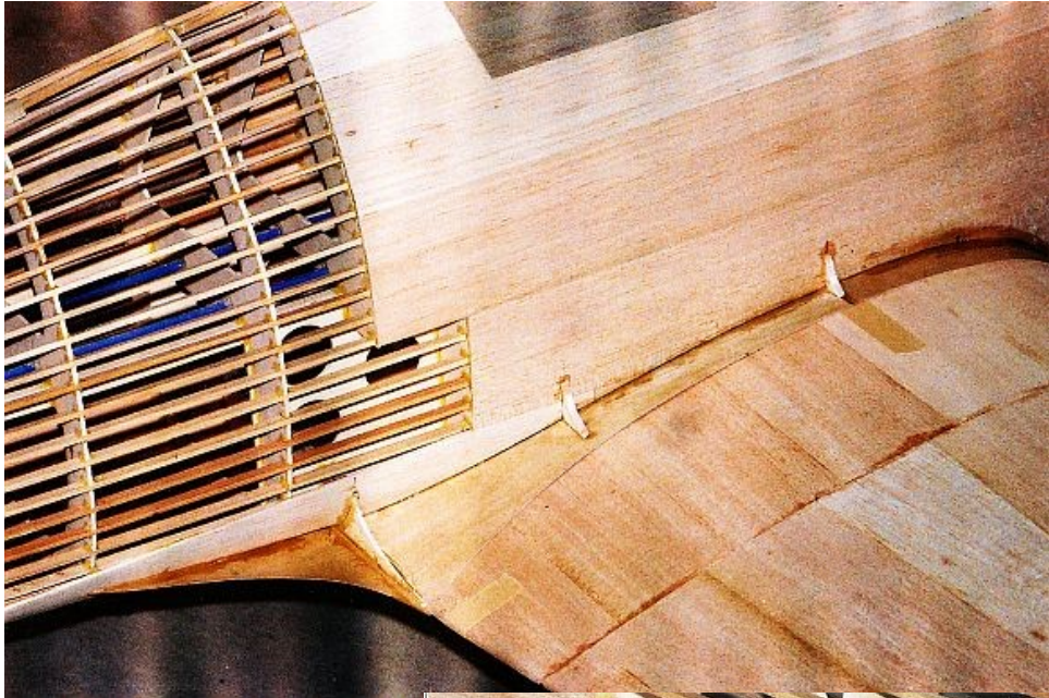
The ply strips are cut to shape and formers for planking are added.
