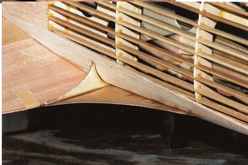
The fairing is planked with balsa to the front former placed about half chord. The balsa needs to be softened by spraying with ammonia to conform with the required curves.
