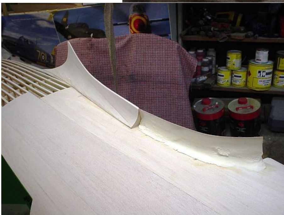
From the front of where the planking ends the fairing is made from a bog of micro balloons and finishing resin.
